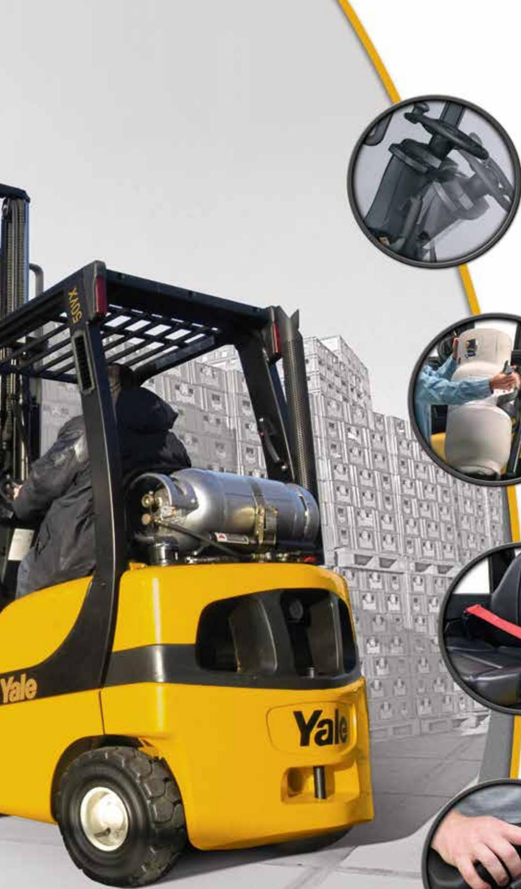
Yale Veracitor® VX forklift design goals include easy entry and exit, superior driver comfort, and ease of operation. The ergonomically designed 12" steer wheel with spin knob and infinitely adjustable steer column are shown.
